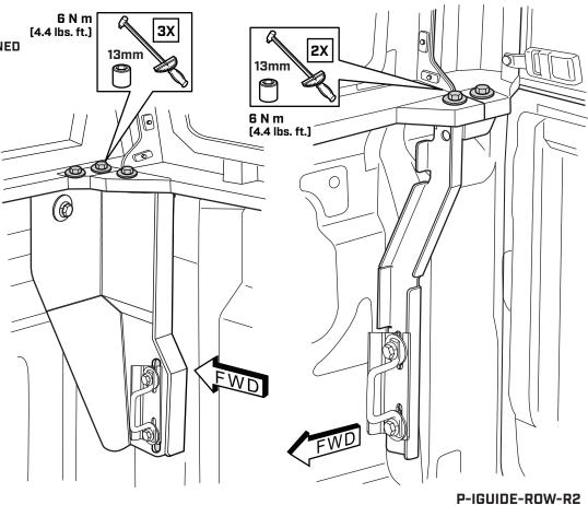
ONCE SMARTCAP IS POSITIONED CORRECTLY, FULLY TIGHTEN LOWER FASTENERS WITH TORQUE WRENCH AS INDICATED.
