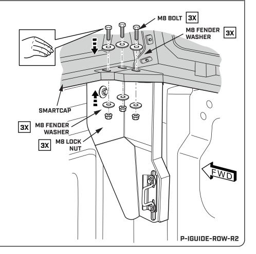
SECURE THE SMARTCAP TO THE RIGHT REAR MOUNTING BRACKET WITH THE FASTENERS AS INDICATED, HAND TIGHTEN ONLY.
