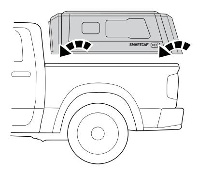
CHECK THAT THE SMARTCAP IS PROPERLY POSITIONED AND CENTERED ON THE TRUCK BED
