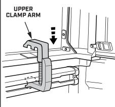
TIGHTEN MOUNTING CLAMPS USING TORQUE WRENCH AND 13MM SOCKET TO 4.4 FT. LBS. (6 NEWTON METERS)
