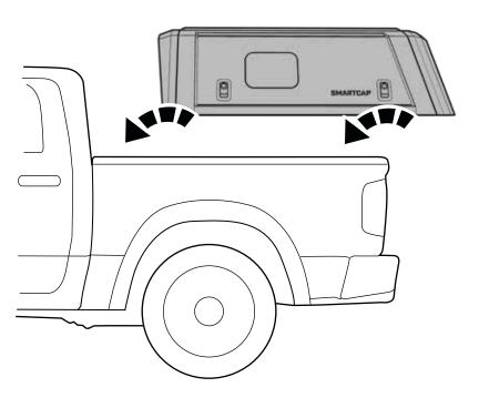
CHECK THAT THE SMARTCAP IS PROPERLY POSITIONED AND CENTERED ON THE TRUCK BED.
