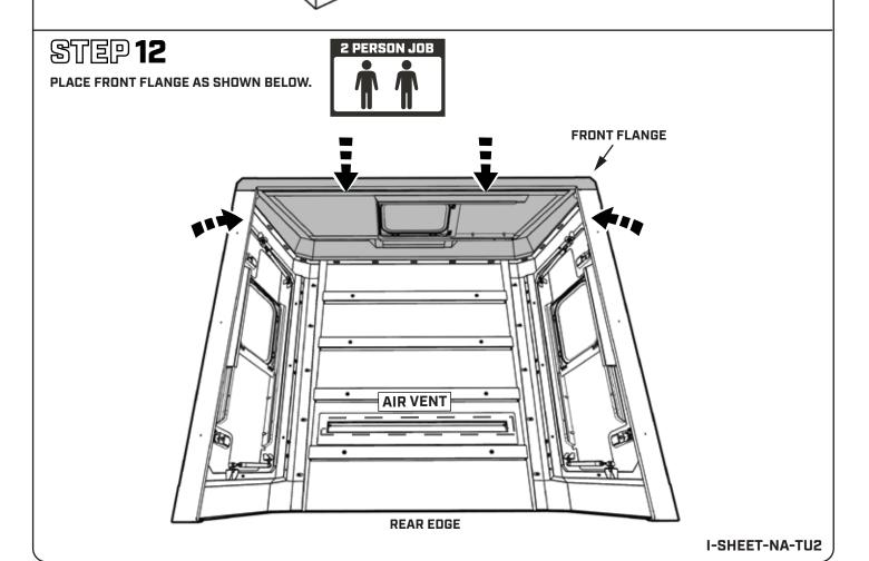
INSTALL HARDWARE ALONG FRONT FLANGE WITH M6 BOLT ON INSIDE.
