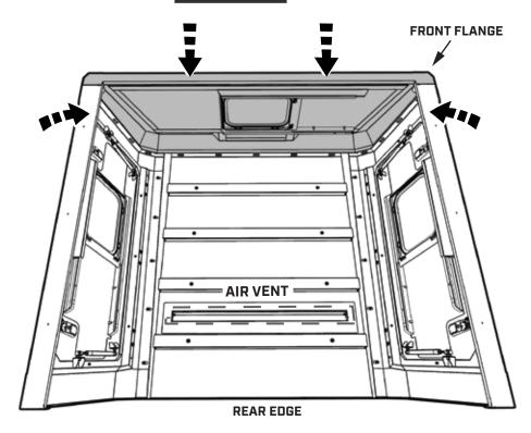
INSTALL HARDWARE ALONG FRONT FLANGE WITH M6 BOLT ON INSIDE.
