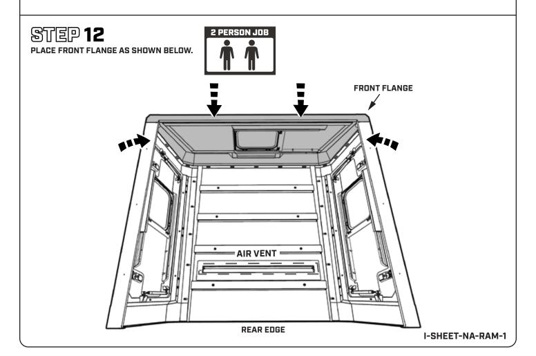
INSTALL HARDWARE ALONG FRONT FLANGE WITH M6 BOLT ON INSIDE.
