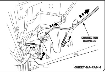
ROUTE THE CONNECTOR HARNESS UP AND OVER THE REAR WHEEL WELL.
